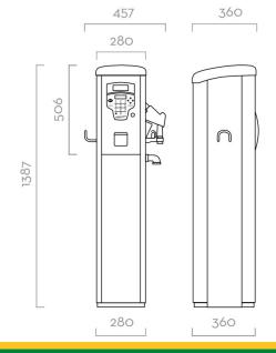
Measurements in millimeters
