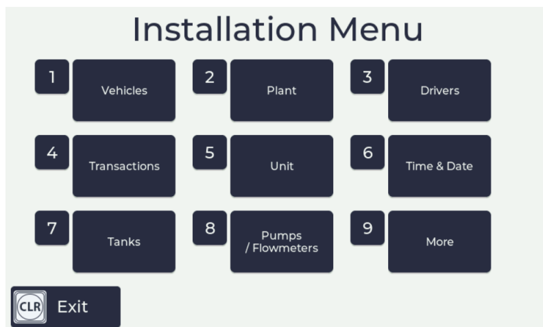
Figure 5.3: Installer Menu with SmartDip fitted
