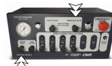
**1** Press down on the "MANIFOLD VALVE" and "TRANSFER VALVES" buttons for three (3) seconds for the Trailer B Swift-Mx Box.
