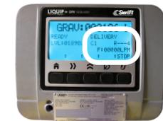
8 Product is dispensed, monitor delivery. **NOTE:** The flow will stop once product in compartment has been delivered or preset is reached.
