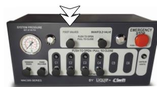
3 Open the foot valves by pressing the "FOOT VALVES" button on the Swift-Mx Box and physically open the first API and product-delivery elbows, as required.
