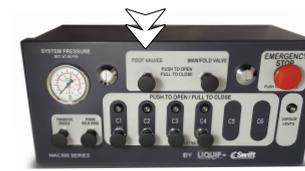
5 Open the foot valves by pressing the "FOOT VALVES" button on the Swift-Mx Box.
