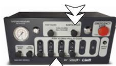
**6** Hold the "MANIFOLD VALVE" and "SELECTED COMPARTMENT" buttons for three (3) seconds.
