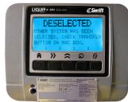
If the DFV-Swift displays "DESELECTED," it means you are using a dual-trailer configuration.
